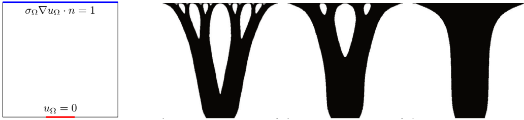
Figure 3.3: Optimal heater: boundary conditions ( \nabla u_{\Omega} \cdot n = 0 when non specified) and optimal designs for increasing values of \eta . Here there is no true volume constraint but a fixed penalty \lambda|\Omega| added to the cost.
